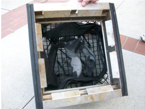
Plastic Netting – poor flow & does not last
